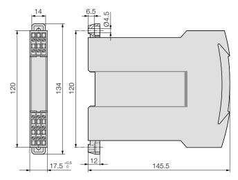
Fig. 10. SINEAX B 811 in housing  $\bf S17$  clipped onto a top-hat rail (35×15 mm or 35×7.5 mm, acc. to EN 50 022).
