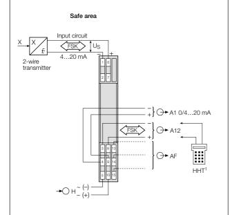
Fig. 6. SINEAX Type 811-1..1 ....., Non-Ex input and output circuits, supply voltage U<sub>S</sub> 24 V DC, designed for FSK.
