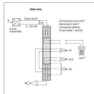
Fig. 4. SINEAX Type 811-1..0 ....., Non-Ex input and output circuits, supply voltage  $U_{\rm S}$  24 V DC, not designed for FSK.
